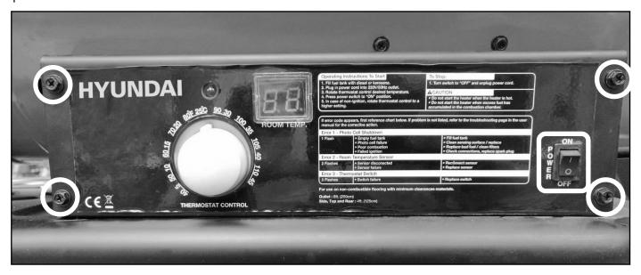
3. With the bolts removed, gently pull the control panel away from the unit body, exposing the control board.
