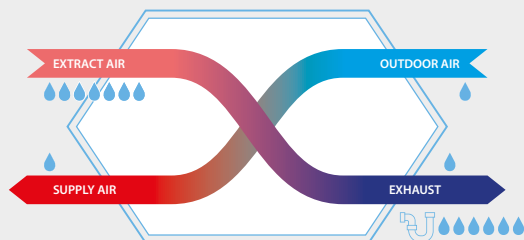
Aluminium and plastic heat exchanger Sensible energy (heat) is recovered from the extract air and transferred to the fresh supply air.
