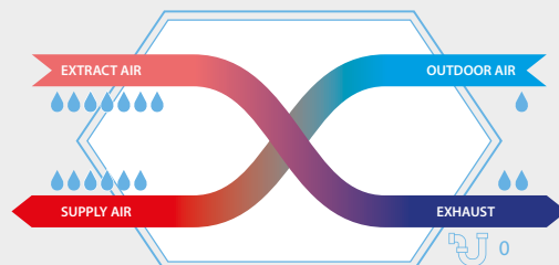
Enthalpy heat exchanger Sensible energy (heat) and latent energy (humidity) is recovered from the extract air and transferred to the fresh supply air.
